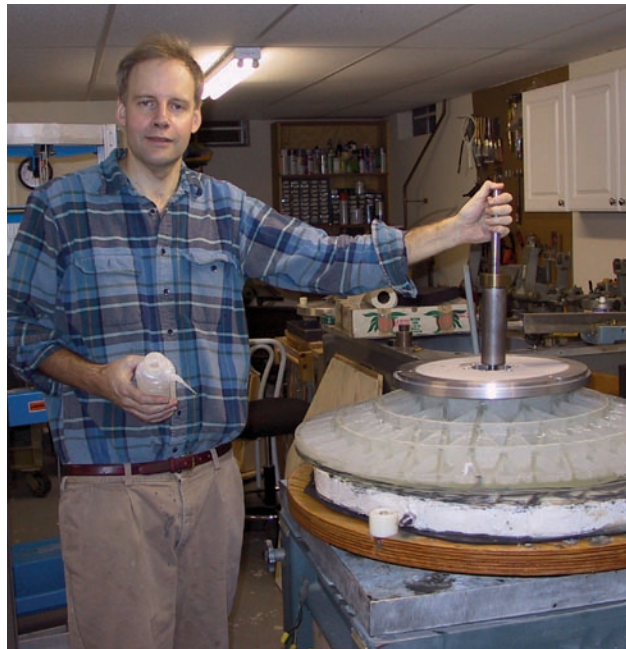
The relay telescope’s novel optical design is the handiwork of Scott Milligan, who also did much of the optical fabrication as “incentive” for the author to select the design for his project. Note the primary mirror’s lightweight structure described in the text.
